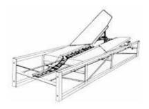
BALE KICKOFF: Sturdy, tapered design provides for fast, smooth, accurate unloading to either right or left from any point along conveyor. Pull control rope (rope not included), from mow floor to change direction of unloading or to slide kickoff to any position along full length of conveyor. Bales cannot be conveyed over kickoff and onward toward end of conveyor.
